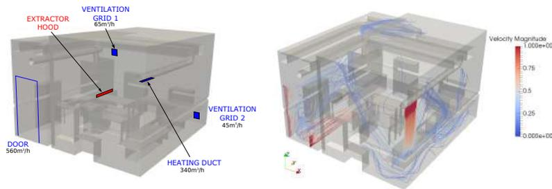
Figure 8: Numerical mock-up of the laboratory room and measured incoming flows (left)
