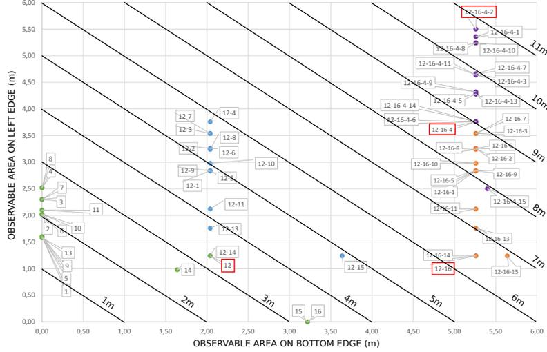
Figure 5: Optimal placement (red rectangles) in the 2D domain of several sensors of with an LOD of  $10\text{ppm}$  - Observable Areas - Isovalues of the total observable area are represented as solid lines
